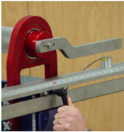
Position Load Cell to desired moment arm dimension from tube centerline (Step 2).
