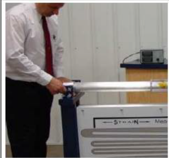
Secure block end with capture knobs while pulling up on cantilever end to remove sag.
