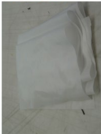
Resin Flow Control: Perforated Release Film
