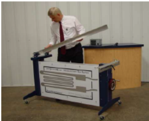
Position I-Beam Assembly Into Frame
