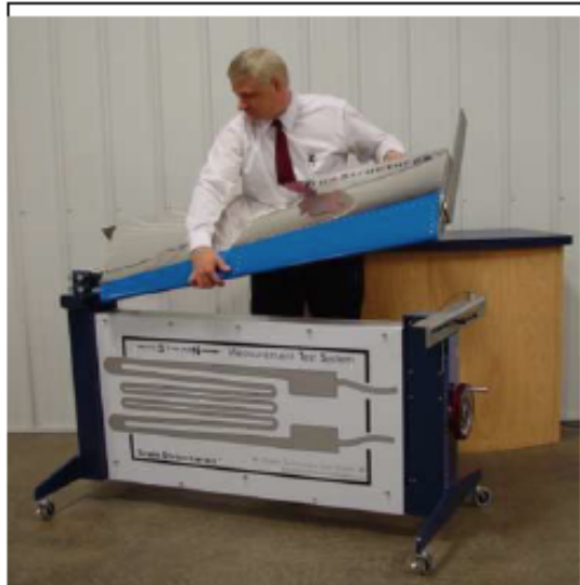
Position wing to align spar ends with fixture tangs.
