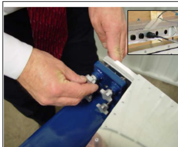
Finger tighten knobs. Lift up on cantilever end of wing to remove any sag in system. Tighten knobs firmly while continuing to lift end of wing. Be sure load cell and strain gage connections to strain bridge controller (data box).
