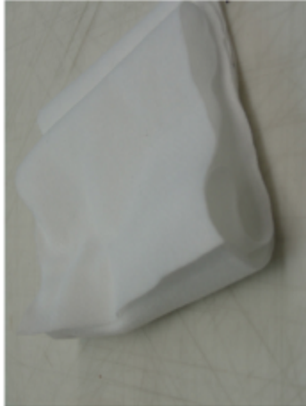
Vacuum Airflow Distribution: Breather Cloth
