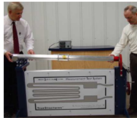
Loosen capture knobs on capture block end and slide tube out of yoke.
