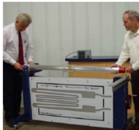
Position tube in cantilever position, tighten hand knobs while pulling up on tube end..
